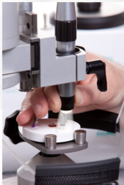
↳ Processing of titanium abutment with laboratory turbine LED Carver and Turbi-Jet
